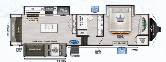
HITCH (LBS.): 2,273 UVW (LBS.): 12,345 CCC (LBS.): 3,928 LENGTH: 37' 4" EXTERIOR HEIGHT: 13' 5" WIDTH: 101" TANKS (F/G/B): 63 / 90 / 45 AWNING: 18' & 10' 6"
