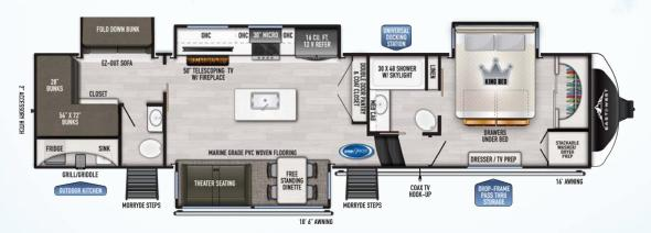
HITCH (LBS.): TBD UVW (LBS.): TBD CCC (LBS.): TBD LENGTH: TBD EXTERIOR HEIGHT: 13'4" WIDTH: 101" TANKS (F/G/B): 63/90/90 AWNING: 16'&10'6"
