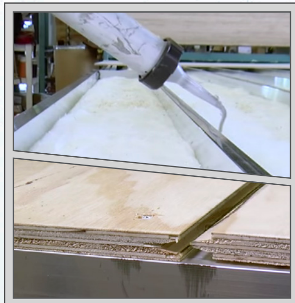
GLUED & SCREWED PLYWOOD FLOORING 5/8" Tongue & Groove Plywood Floors Glued & Screwed on Aluminum Floor Joist (16" on Center)
