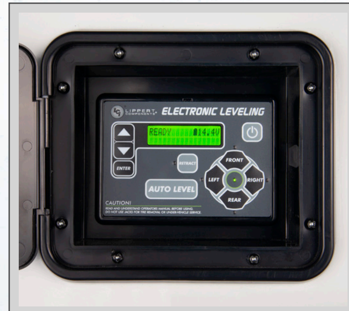
AUTOMATIC LEVELING SYSTEM 6-Point Hydraulic Automatic Leveling System
