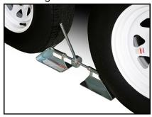
Press **ON/OFF** to activate display. Press **LANDING GEAR MODE**. Press and hold **EXTEND** until the necessary detachment height is reached. Disconnect, and pull the tow vehicle completely clear of the unit. Lower the rear leveling jack adjustable feet and position them so that they are close to the same distance from the ground. Press **AUTO MODE**.
