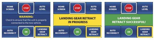
Raise all adjustable feet to the hole that provides the most ground clearance before towing the unit. Press **ON/OFF** to deactivate the display. **WARNING:** Visually check all jacks to ensure that they are fully retracted before towing the unit.
