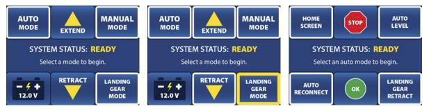
Press **OK** to begin "LANDING GEAR RETRACT" or **STOP** to make another selection. The display will read "LANDING GEAR RETRACT IN PROGRESS". When the jack has been fully retracted the display will read "LANDING GEAR RETRACT SUCCESSFUL" and a beep will sound. If the "LANDING GEAR RETRACT" does not fully retract the jacks, simply repeat the "LANDING GEAR RETRACT" process, or use "LANDING GEAR MODE" to finish retracting the landing gear.
