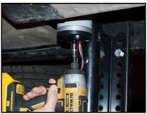
**Landing Gear** – Using the manual crank handle, alternately crank each landing gear jack a few turns at a time to raise or lower the landing gear.
