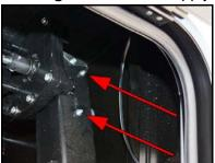
Rear Leveling Jacks – With the jack extended half way remove the plastic plug and apply
