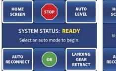
The system will go through a series of moving the jacks and checking the unit for level. The display will read "AUTO LEVEL IN PROGRESS". When the system has successfully leveled the unit, the display will read "AUTO LEVEL SUCCESSFUL" and a beep will sound.
